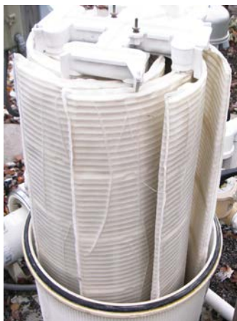
Same filter after chemical cleaning
